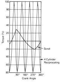
Chart illustrates low torque variation of 3-D Scroll compressors reciprocating compressor.
